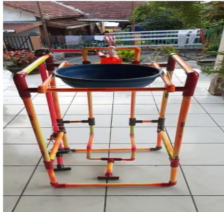
Gambar 9. Alat Cuci Tangan Injak
